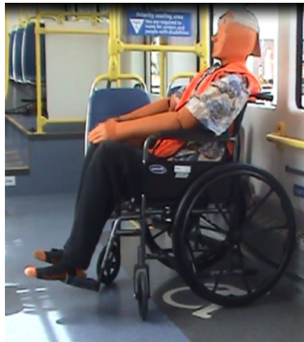
FIGURE 3. Side-facing occupied manual wheelchair on light rail vehicle
